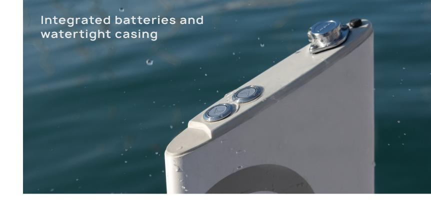
Integrated 1085 Wh battery is fully protected from all weather conditions and contains enough juice to get you more than 14 miles of range at a 3 mph cruising speed on a tender boat.
